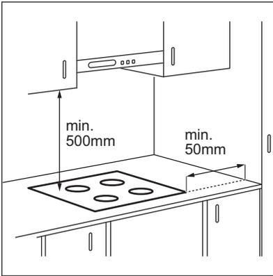
If the appliance is installed above a drawer, the hob ventilation can warm up the items stored in the drawer during the cooking process.
