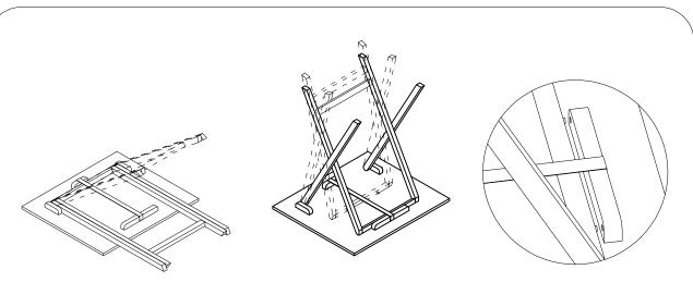
Warning - Please ensure that the wooden locating pins are in position before using the table.
