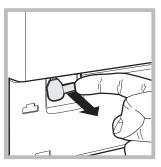
4. pull outwards using the tab as indicated in the figure, until the plastic tie-rod is freed from its stop position; pull downwards until you hear a "click", which indicates that the door is now unlocked.
