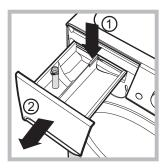
To remove the drawer, press lever (1) and pull the drawer outwards (2) (see figure). Wash it under running water; this procedure should be repeated frequently.
