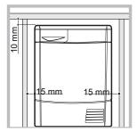
Install the dryer far from gas ranges, stoves, radiators or hobs as flames may damage it. If the dryer is installed below a worktop, ensure there are 10 mm between the upper panel of the dryer and any objects above it and 15 mm between the sides of the machine
