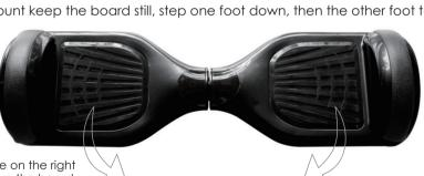
Increased pressure on the right foot plate will move the board forward by turning left
