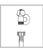
1. Connect the supply pipe by screwing it to a cold water tap using a <sup>3</sup>/<sub>4</sub> gas threaded connection (see figure).
