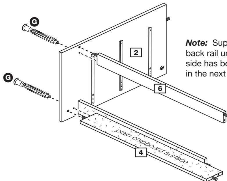
**Note:** Support the back rail until the left side has been fitted in the next step.
