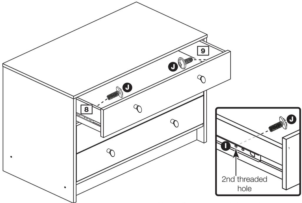
**Note:** Do not overtighten the screws. If they catch on the runner you may need to loosen them slightly.
