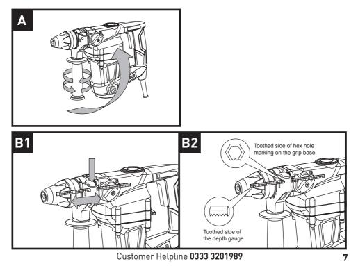
into the handle. Slide the depth gauge until the distance between the depth gauge end and the drill bit end is equal to the depth of hole/screw you wish to make.. Release the locking button to tighten.
