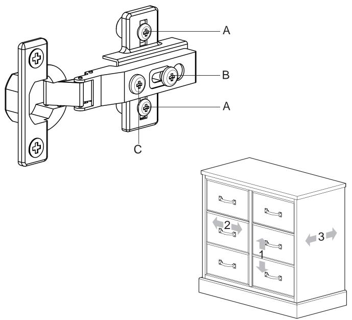
3. To adjust the distance away from the unit loosen screw 'B', this allows the hinge arm to slide back and forth. Adjust as required then re-tighten screw 'B'.
