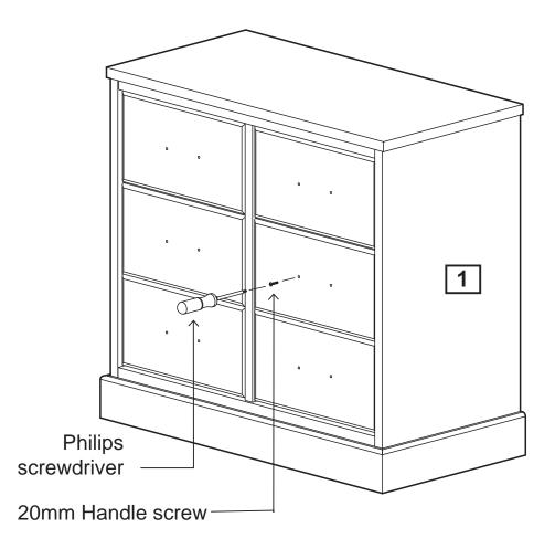
**b:** Replace the D handle on the front of the unit. Fix in position by screwing the 20mm handle screw into each D handle from inside the unit using a Philips screwdriver.
