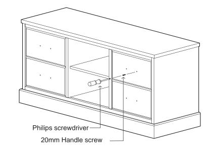
**b:** Replace the D handle on the front of the unit. Fix in position by screwing the 20mm handle screw into each D handle from inside the unit using a Philips screwdriver.
