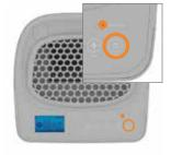
Plug the appliance into a power source and press the on button. Insert a small blunt instrument such as pen nib into the reset insert and hold down for a few seconds to reset the filter life calculator. A beep sound will be heard to confirm the filter reset has been set and the LCD screen will turn blue again.
