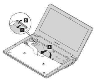
**6** Reinstall the new keyboard and tighten the screws.
