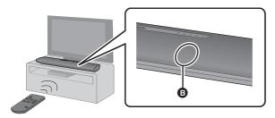
B Remote control signal sensor
