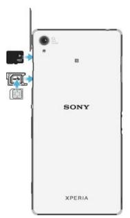
Make sure you insert the nano SIM card into the nano SIM card holder before inserting it into the device. Also, don't confuse the nano SIM card slot with the memory card slot.
