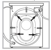
3. Remove the protective screws (used during transportation) and the rubber washer with the corresponding spacer, located on the rear part of the appliance (see figure).
