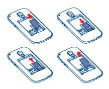
Place the SIM card with the chip facing downwards and slide it into its housing. Make sure that it is correctly inserted. To remove the card, press and slide it out.
