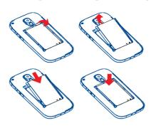
Insert and click the battery into its place and close the telephone cover.
