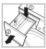
To remove the drawer, press lever (1) and pull the drawer outwards (2) (see figure).
