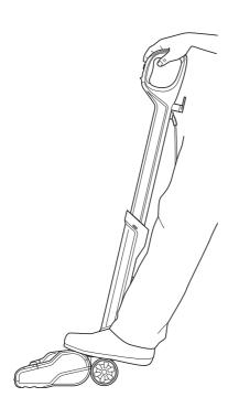
Stand the vacuum upright. Step on the Motorised Floor Nozzle and pull the 1 Wand back to start vacuuming.
