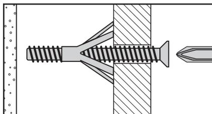
For use with plasterboard partitions or hollow wooden doors.
