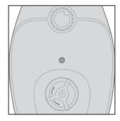
2. Plug into mains, turn dial to 'ON'; the amber light will illuminate to indicate power on. The steamer will be ready after approximately 30 seconds.
