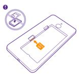
**5.** If you have a memory card, push the card into the memory card slot. It is recommended that you use a fast microSD card from a well-known manufacturer.
