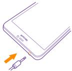
Do not connect to products that create an output signal, as this may damage the device. Do not connect any voltage source to the audio connector. If you connect an external device or headset, other than those approved for use with this device, to the audio connector, pay special attention to volume levels.
