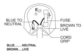
• Under no circumstances should Neutral or Live wires be connected to the 'E' (Earth) terminal.
