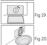
3.Reinstall each part back after sundries matters are removed (Fig20).
