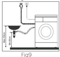
Important: Drain hose can be fitted to the drainer or a wash basin.
