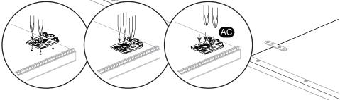
**g:** Underside. Mount 2x back guide part (A), each with 2x screws (AC) on segment [1].
