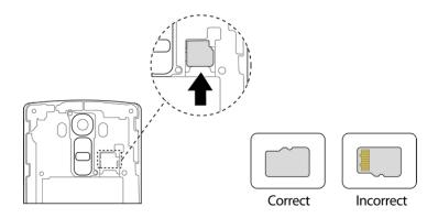
• Insert the microSD card all the way gently without bending and with the terminals facing down.
