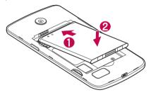
4 To replace the cover onto the device, align the back cover over the battery compartment 1 and press it down until it clicks into place 2.
