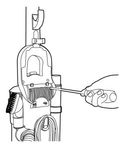
Screw handle in place with the screws provided.
