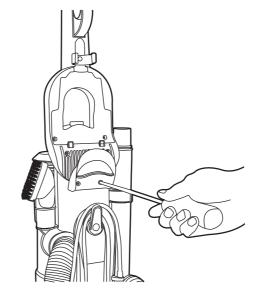
Attach and screw hose hook in place.
