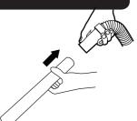
Check the hose by removing it from the cleaner, stretching it to full length.
