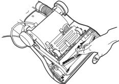
Remove brush assembly and check for wear on the belt. Loop the new belt around the motor and brush channel.
