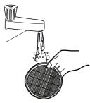
Wash the filter under hand warm water until the water runs clean. Remove excess water by shaking and leave to dry for 24 hours. When completely dry reassemble and refit filters to cleaner.
