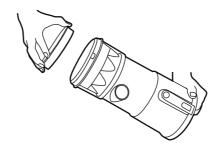
Remove the filter assembly from the dust bin.
