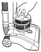
1 Remove the dust container rotate and remove the exhaust filter cover.
