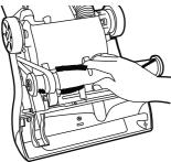
Refit the brush guard with 5 retaining screws.
