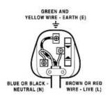
The wires in this mains lead are colored in accordance with the following code:
