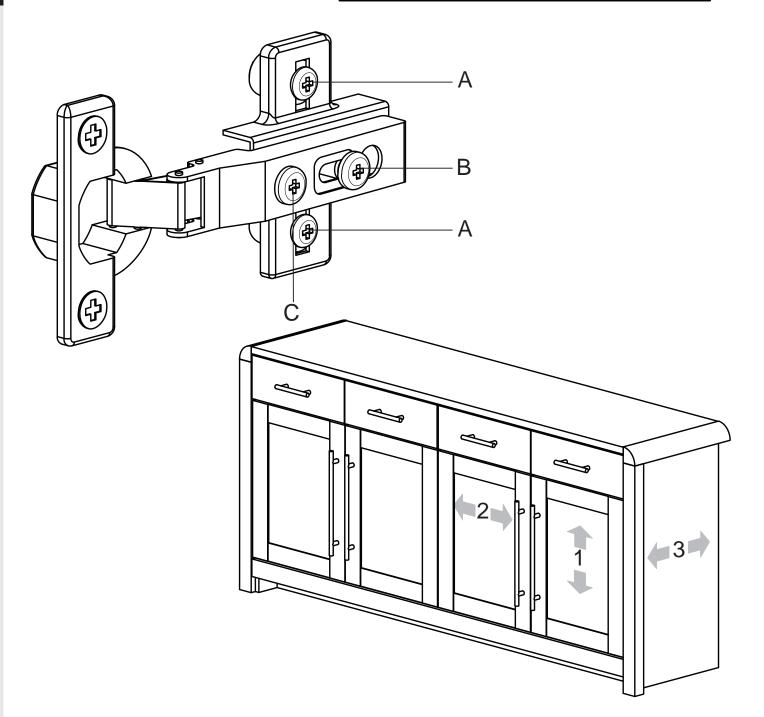
3. To adjust the distance away from the unit loosen screw 'B', this allows the hinge arm to slide back and forth. Adjust as required then re-tighten screw 'B'.
