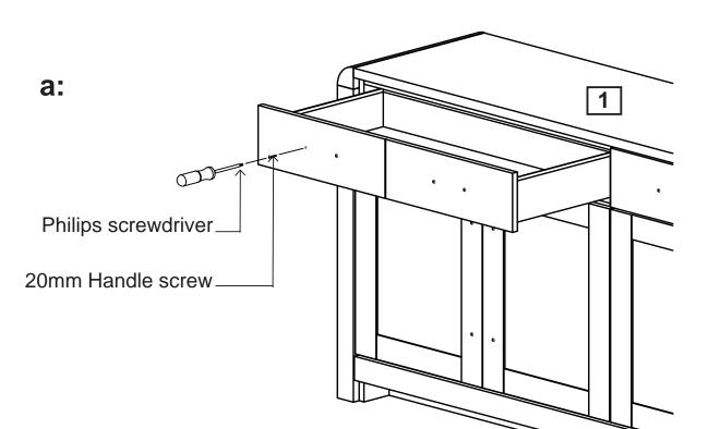
**b:** Replace the large and small bar handle on the front of the unit. Fix in position by screwing the 20mm handle screw into each bar handle from inside the unit using a Philips screwdriver.
