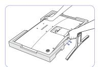
While holding the upper part of the monitor with one hand, pull the stand neck with the other hand in the arrow direction to detach the stand.
