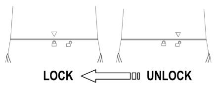
Turn clockwise to lock the goblet onto the motor unit
