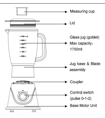
**WARNING**: The Jug Base and Blade Assembly are permanently fixed to the glass jug at ex-factory. DO NOT ATTEMPT TO REMOVE THE JUG BASE FROM THE GLASS JUG. It would damage the product permanently.
