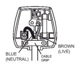
The wires in this mains lead are coloured in accordance with the following code:
