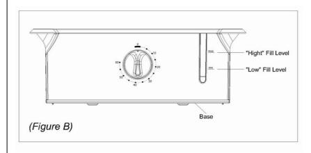
The high fill level is for long time cooking while the low fill level for shorter time.
