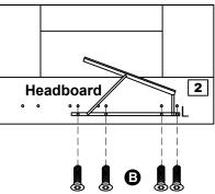
Footboard fixing holes position for left side opening
