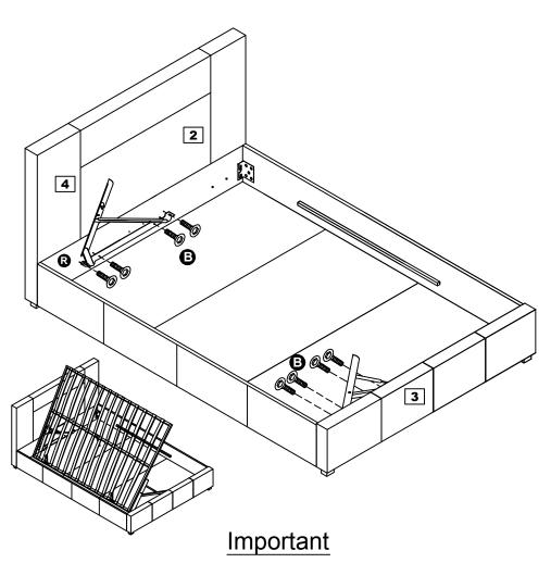
Headboard fixing holes position for right side opening
