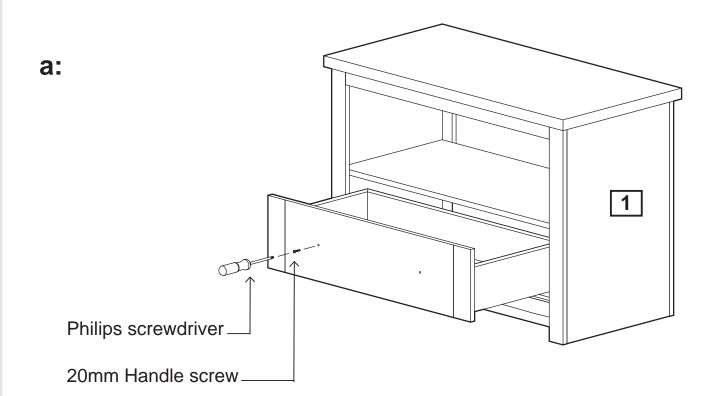
**b:** Replace the knob handle on the front of the unit. Fix in position by screwing the 20mm handle screw into each knob handle from inside the unit using a Philips screwdriver.
