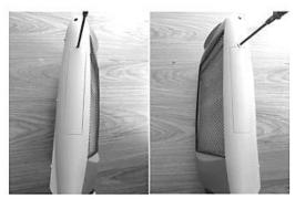
2. Use pliers to clamp the internal lock of latch.
