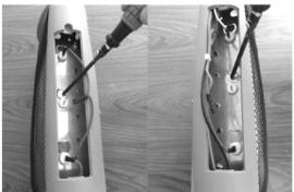
Reconnect the wires to the tube terminals on both sides.
