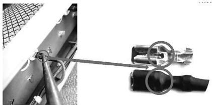
3. Disconnect the wires from the tube terminal on both sides.
