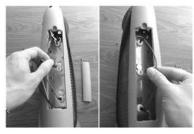
4. Open the tube holders on both sides.
