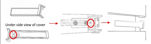
3. On the second fastening connecting bracket on the opposite side, you simply just have to slot the hinge cover on to it via the clips.
