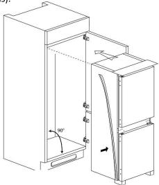
Open the door and push the side of the appliance without the hinges against the side of cabinet wall. Fix the appliance in two places, 4 round headed screws in the top plinth at the top of the appliance and the 2 large screws in the foot at the bottom of the appliance that does not hinge the freezer door.
