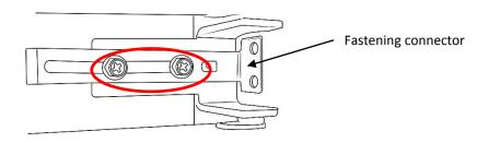
2. Slot on the hinge cover, the 2 clips on the back of the cover should slot into the raised clip on the fastening connector
