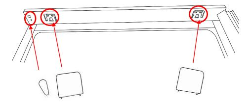
Apply a blanking cover by clipping it in to place on the foot at the bottom of the appliance that does not hinge the freezer door.
