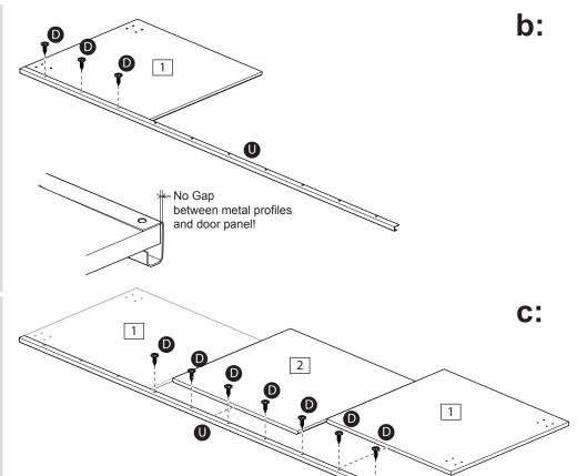
**C:** Mount segment middle 2 with 3x screws **D** on door trim **U**. Mount segment 1 with 4x screws **D** on door trim **U**.
