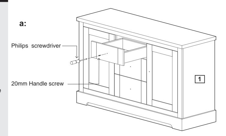
**b:** Replace the knob handle on the front of the unit. Fix in position by screwing the 20mm handle screw into each knob handle from inside the unit using a Philips screwdriver.
