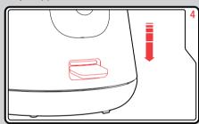
Press the On/Off Switch (6). The Switch will Illuminate.
