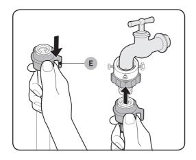
**7.** While holding down part (E), connect the water hose to the adaptor. Then, release part (E). The hose fits into the adaptor with a clicking sound.
