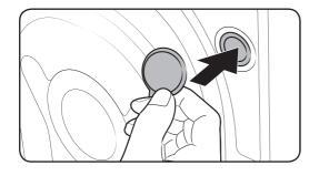
**1.** Fill the holes with the supplied plastic bolt caps.
