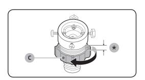
**4.** Hold the adaptor and turn part (C) in the arrow direction to loosen it by 5 mm (\*).
