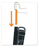
Slide the handle down onto the main body of the unit.
