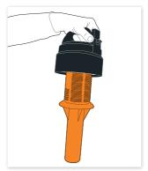
Wipe the separator with a cloth to remove any dirt.
