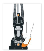
Place foot on the vacuum to recline the vacuum body as desired.
