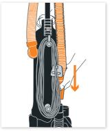
Insert the lower hose to the lower hose connector.
