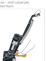
Place foot on the on/off button to switch the vacuum cleaner on.
