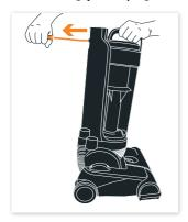
Using a crosshead screwdriver, remove the screw from the back of the unit as shown.
