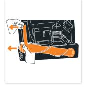
Lift the brush bar out of the base of the unit. Next, remove the belt from the brushbar and from the motor spindle towards the rear of the floor head. Replace the belt.
