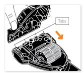
To re-assemble the TurboTool, ensure that the tabs are engaged and pivot the lower housing closed. Slip the locking ring over the neck of the TurboTool and into the groove to secure.
