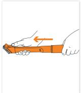
**IMPORTANT:** When the vacuum cleaner is stood in the upright position, or when using the hose and tools, the brush bar height adjust must be set to the highest position.
