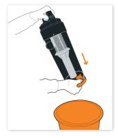
Hold dirt container over a bin and press the dirt container latch to open, allowing dirt to fall out.
