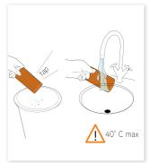
Tap the HEPA central filter against a bin and wash it under running water (max 40°c. Dry thoroughly (24 hrs) before returning filter to the unit.
