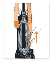
Pull out the lower hose from the lower hose connector.
