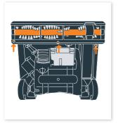
Turn unit over and remove the three screws using a crosshead screwdriver as indicated by arrows.
