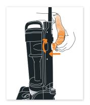
Connect the upper hose to the upper hose connector, rotate hose clockwise to secure.
