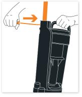
Return the screw and tighten, securing the handle into the main body of the unit.
