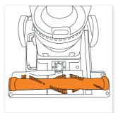
Once the belt has been replaced attach the brushbar back onto the vacuum.
