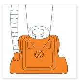
Attach the floorhead cover, 2 small wheels and height adjuster dial by screwing back into place.
