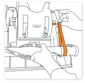
Place the belt by attaching it to the brushbar and hooking it onto the metal side.
