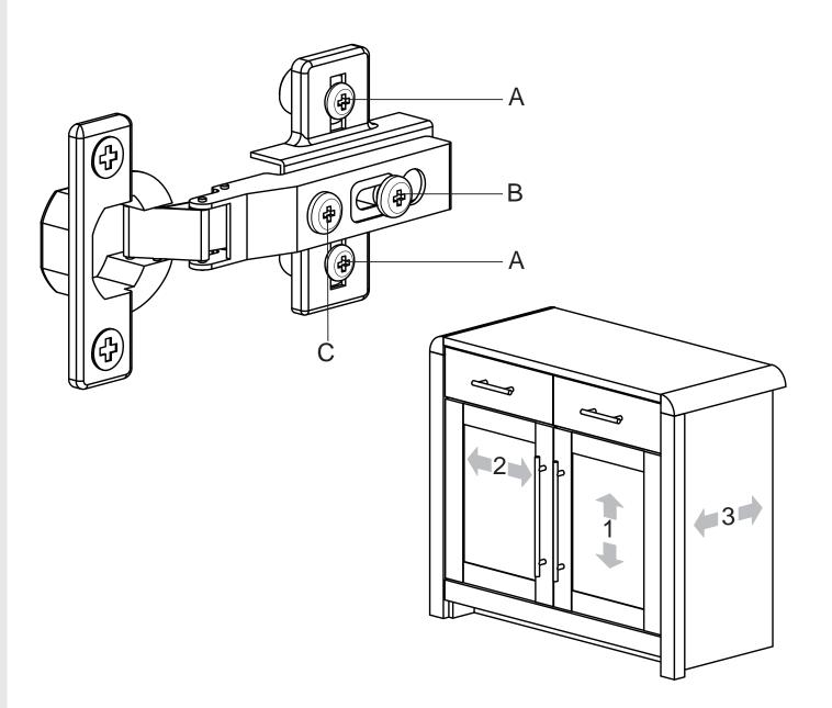
3. To adjust the distance away from the unit loosen screw 'B', this allows the hinge arm to slide back and forth. Adjust as required then re-tighten screw 'B'.
