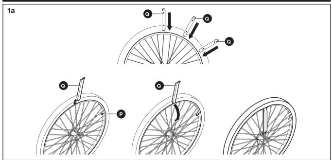
If you have a puncture, you will need to remove and repair the inner tube.
