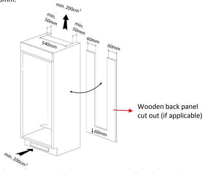
Carefully push the appliance into the housing, ensuring that the cabinet doors are able to fully close.
