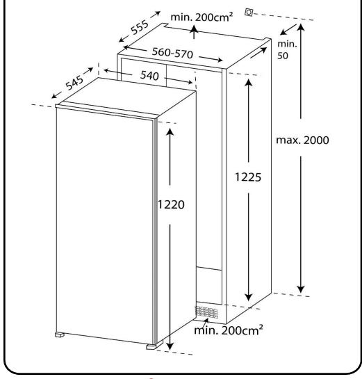
The cabinet in which the appliance is housed in must have a ventilation recess of  $(W)540 \times (D)50mm$ .
