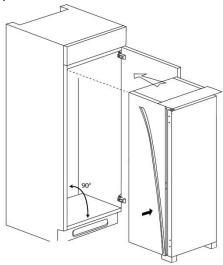
Open the door and push the side of the appliance without the hinges against the side of cabinet wall. Fix the appliance in two places, 4 round headed screws in the top plinth at the top of the appliance and the 2 large screws in the foot at the bottom of the appliance that does not hinge the door.
