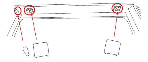
Apply a blanking cover by clipping it in to place on the foot at the bottom of the appliance that does not hinge the door.
