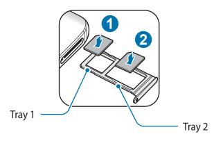
4 Gently press the SIM or USIM card into the tray to secure it.
