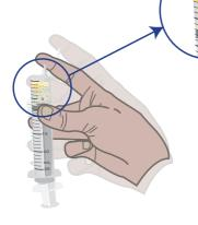
4 Put your finger over the nozzle of the syringe and shake! Keep going until the card breaks down into fibres, and then gently but firmly squeeze the liquid from the syringe back into the little cup.
