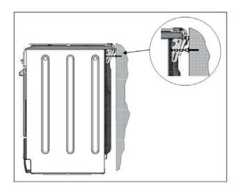
! In order to prevent accidental tipping of the appliance, for example by a child climbing onto the oven door, the supplied safety chain MUST be installed!
