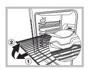
**WARNING!** The oven is provided with a stop system to extract the racks and prevent them from coming out of the oven (1).
